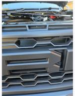
6- Feed LED wire into the 4mm hole.
